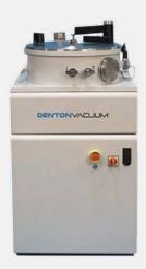
The **Voyager PE-CVD** uses a RF capacitively coupled source for DLC coatings. An optional proprietary chamber configuration is available to enable co-sputtering of metals during diamond-like carbon (DLC) deposition for metal doped DLC (Me-DLC) films.
